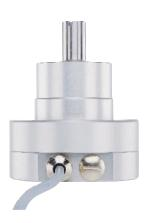
DEIF's rudder/azimuth angle transmitters convert the rudder or azimuth thruster's position angles into either electrical 4-20 mA signals or digital data values with a 16 bit resolution (+/-180de.g. = +/-32767).
