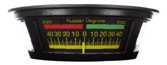
TRI-2 is applied for the indication of the rudder position on the bridge. The indicator consists of a robust moving coil system equipped with 3 pointers mounted on a common shaft. It is suitable if you require analogue input. For CAN input, please refer to the TRI-2 with CAN interface.
